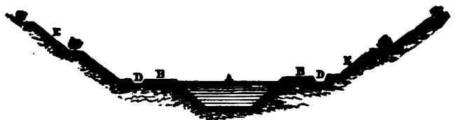
Fig. 166—Cross section of a canal in deep cutting. E, side slopes of cutting.
